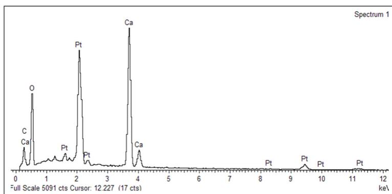
Figure 3. EDX spectrum of commercial calcium peroxide
