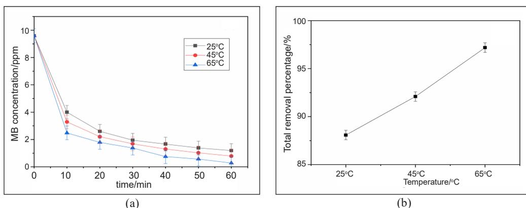
Figure 8. (a) Degradation of the MB concentration over time on the different temperatures at  $25^\circ\text{C}$ ,  $45^\circ\text{C}$ ,  $65^\circ\text{C}$ . (b) Effect of different temperatures on removal of MB (Initial MB concentration = 10 ppm, pH=3.0, 150 rpm, Time = 60 min)
