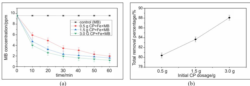
Figure 6. (a) Degradation of the MB concentration over time on different initial dosages in the range of 0.5 g to 3.0 g. (b) Effect of  $CaO_2$  dosage on the removal of MB (initial MB concentration = 10 ppm, Temperature =  $25 \pm 2^\circ C$ , 150 rpm, Time = 60 min)
